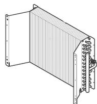
Copper-aluminum evaporator coil, with anticorrosive cataphoresis treatment, with flag-opening baffle on hinges, for cleaning
