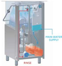
Stabilized pressure rinsing and constant boiler water temperature of 85°C. Thanks to the atmospheric boiler, mixing of mains water in the rinse phase is avoided. The PLUS system also ensures greater control and correct dosing of rinse aid in each cycle.
