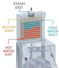
RT system to recover the steam produced by the running machine to preheat the cold feed water. Immediate savings on energy consumption and improved temperature in the working environment, which is no longer saturated by moisture produced by the machine.
