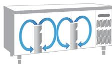
Evaporators placed behind each door pillar to ensure uniformity in cold distribution.
