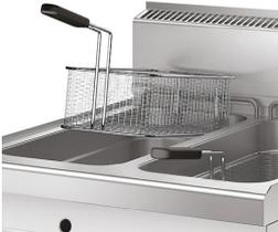
In the gas fryer, the burner is external to the tank and is made of stainless steel with a stabilised flame. Piezo ignition and safety ensured by valve with thermocouple and pilot flame.
